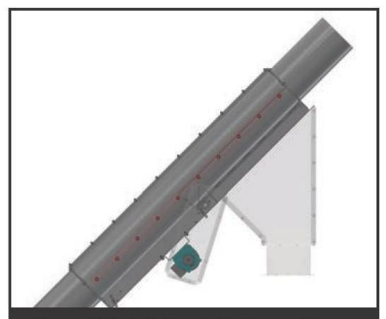
Intermediate inlet and discharge. The Brock GrainDrive Tube Conveyor can easily be configured for multi-bin grain systems. It features modular intermediate inlet and discharge sections. Unlike typical designs, Brock discharges feature roller bearings for easy movement and jam-free operation.
